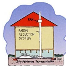
Sub-Membrane Depressurization Sub-Membrane Depressurization
